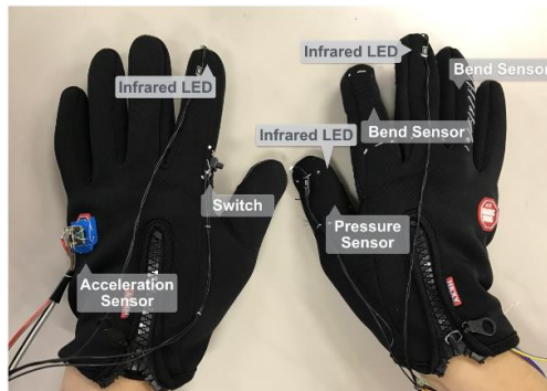
Fig. 7. Glove type device
