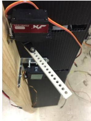
Fig. 4. Servo motors that are attached stock case
