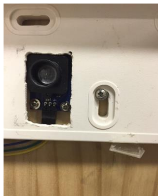
Fig. 2. The color sensor
