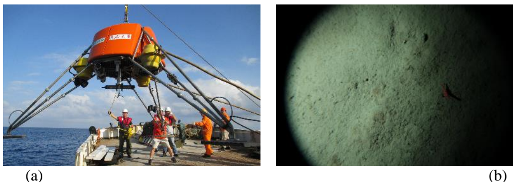
Fig.2 Free-ascending tripod for the seafloor observation in the South China Sea. (a) Loading the equipment. (b) Captured deep sea image.
